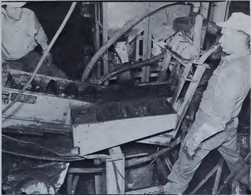
Figure 89.—Laboratory model of spiral-type heavy media separator used for beneficiating aggregates. Lightweight particles are floated off over the weirs shown in foreground and are wasted. Heavy particles sink to the bottom of the heavy media pool, are reclaimed by the spiral, and reworked to remove media. PX-D-14646.
